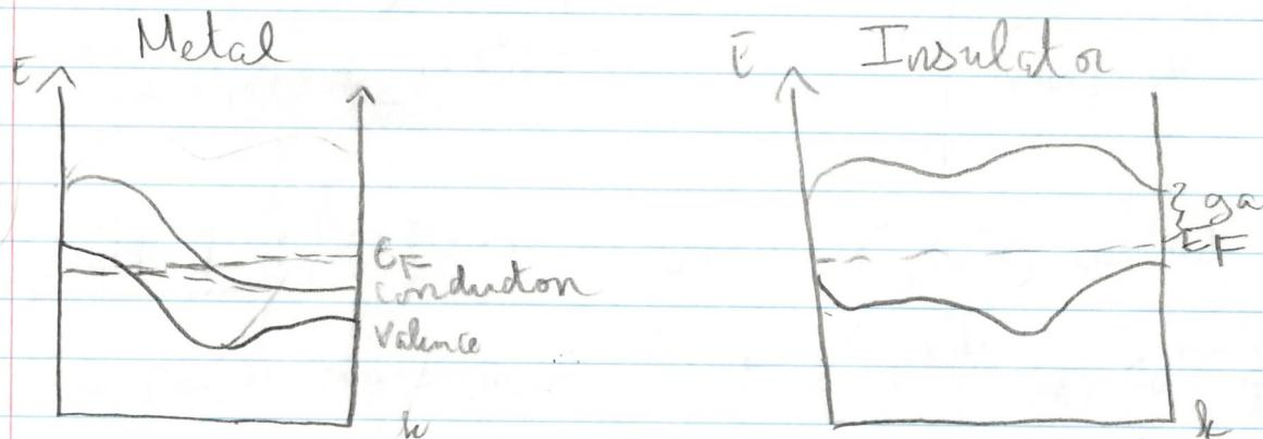
The lack of a gap between valence & conduction band means states are extended.
